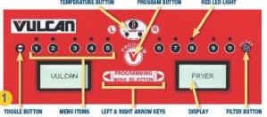
Make sure that the Power Switch is in the "ON" position. Fryer must have power to operate the motor/pump. Fryer Temperature should be between 300-350 Degrees Fahrenheit. RECOMMENDED: ADD OIL TREATMENT MEDIA.
